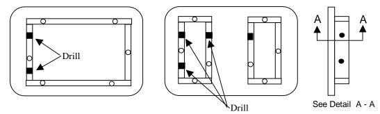
Two  $\frac{1}{4}$ "-20 x 2" carriage bolts are used to provide the beginning of the electrical circuitry. Thread nuts down against the shoulder of two bolts followed by a washer. They are then pressed through the holes drilled in the base frame. This will become the rear of the unit. Place another washer on the bolt followed by another nut. Tighten the nut down very snug so that it will not turn later when the wires are added on the inside and tightened. (See Figure # 2 and Detail A-A above.)
