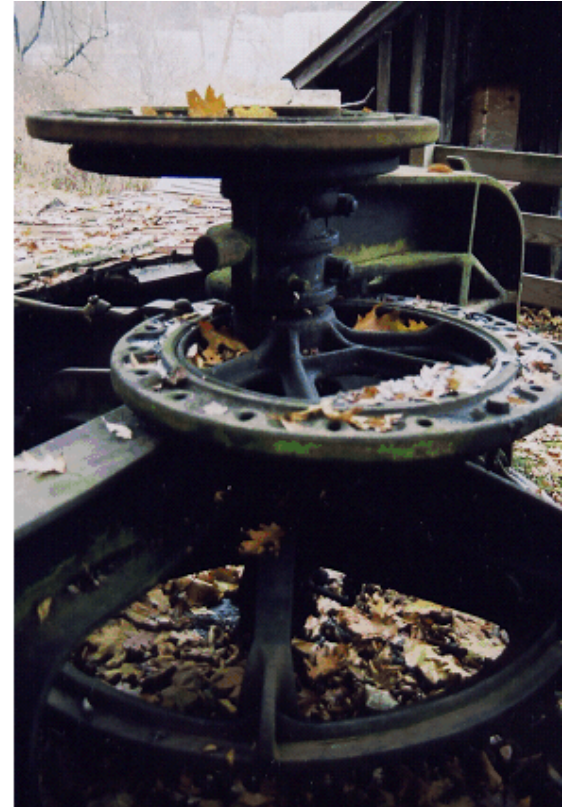
The eccentric gears of the central power pump the line jacks on the wells of the McClintock farm. They run with a Reid engine and are still operational. Photo: K. J. Flaherty, November 2002.
