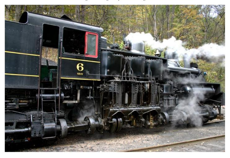
Shay # 6, a Class C-150 three - truck shay weighing in at 162 tons and the last Shay ever built, prepares for the morning run up Back Allegheny Mountain to Bald Knob on October 16, 2005. She is the largest surviving Shay locomotive in the world.
