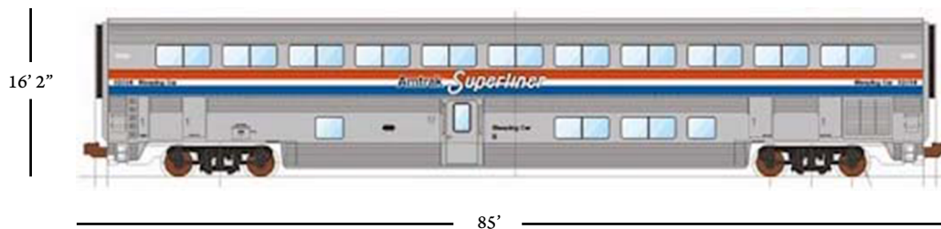
Superliner - Side View Maximum Capacity 44
