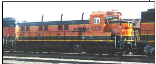
Genset Loco at the Saginaw Yard. Photo by Dusty Garison
