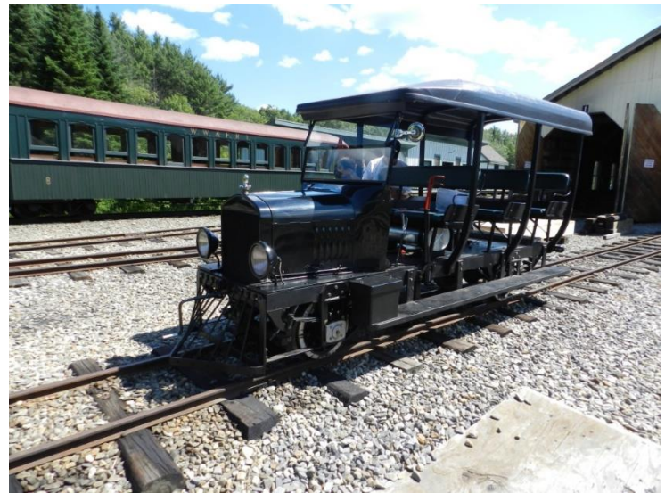
Operational Model T Railcar. This car has a center plate which can be lowered to raise the car so it can be turned 180 degrees.
