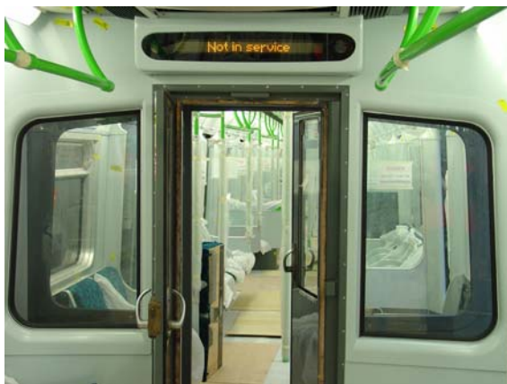
Fig 8 – Car end windows & new PIS pod
