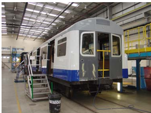
Fig 4 – UNDM car showing new car end windows
