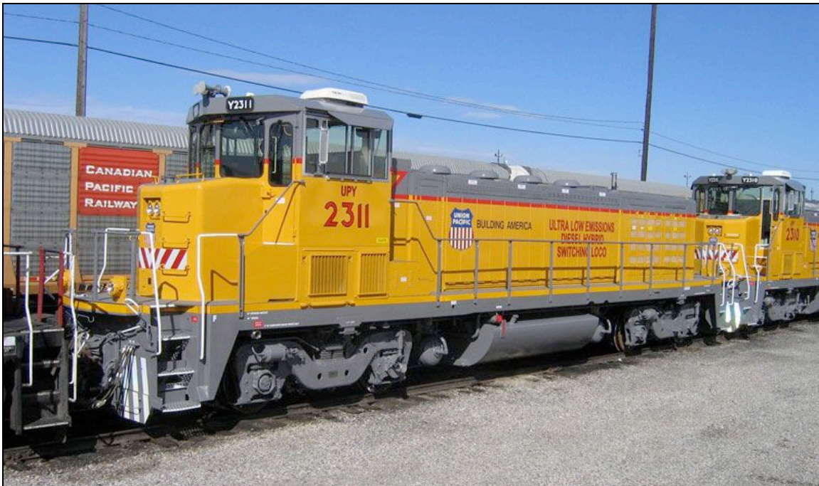
Figure 7 , UPY 2311 and 2310 (GG20B ph III on GE frame).
