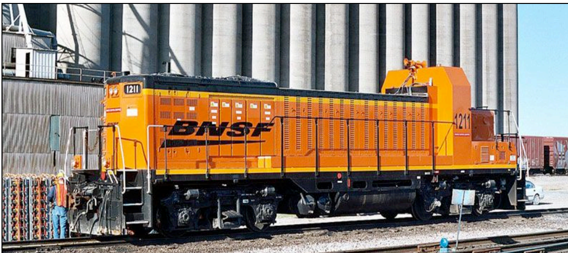
Figure 5, BNSF 1211 (GG20B ph II without cab).
