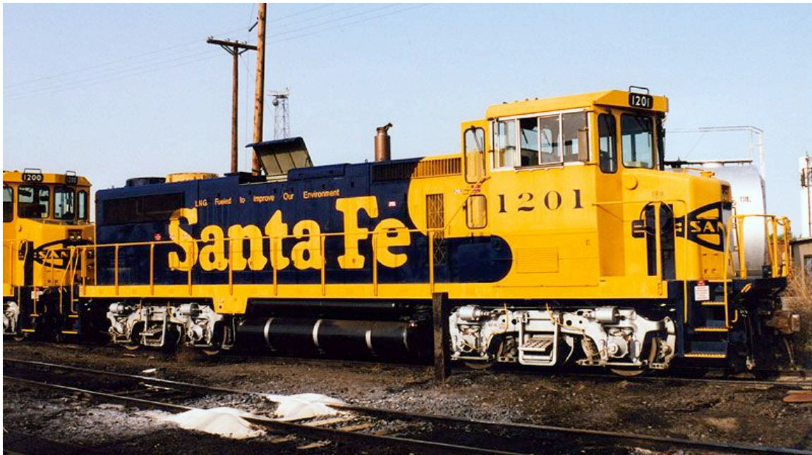
Figure 24 , ATSF1201 (LNG-powered MK1200G).
