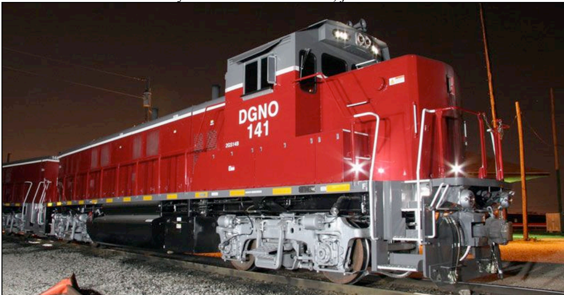
Figure 19 , DGNO 141 (NRE 2GS14B on new frame).
