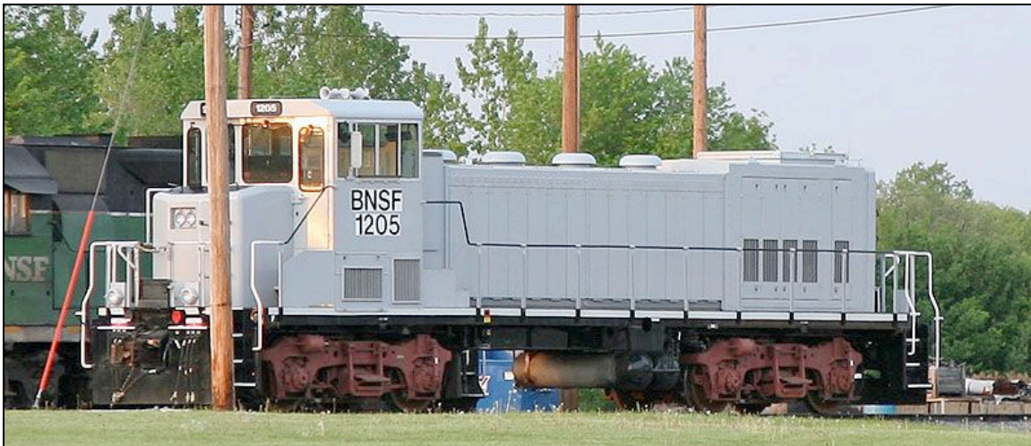
Figure 5, BNSF 1205 (Fuelcell GG20B, incomplete).
