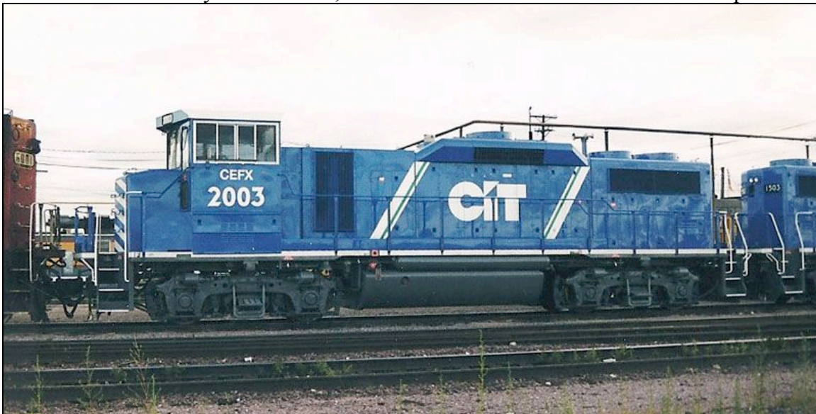
Figure 26 , CEFX 2003 (EMD/MPI GP20D with dynamics).
