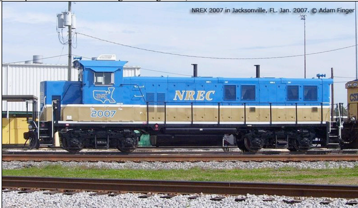
Figure 18 , NREX 2007 (NRE 2GS14B on EMD frame).
