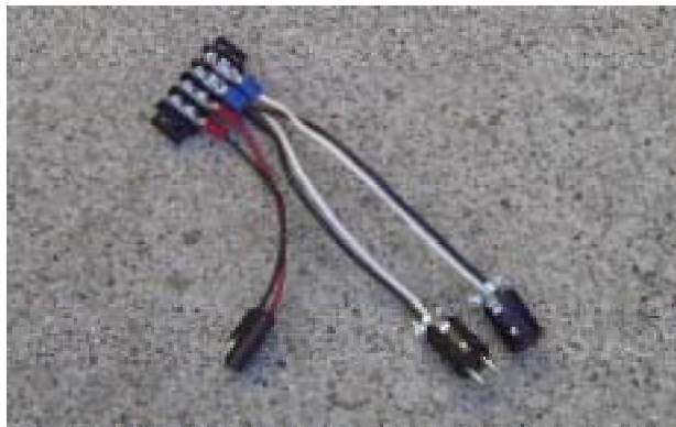
A typical pig-tail for Track and Accessory busses.
