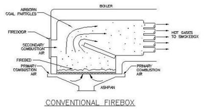
firebox through holes in the firedoor, and sometimes through openings installed in the sides of the firebox (such as over-fire jets).
